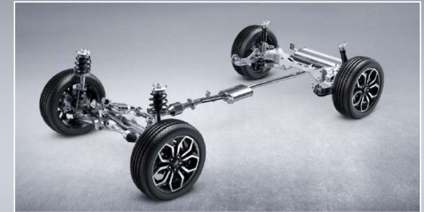
LEADING DRIVING COMFORT IN ITS CLASS The X50 is equipped with a rare combination of front MacPherson and rear multi-link independent suspension systems in its class.
