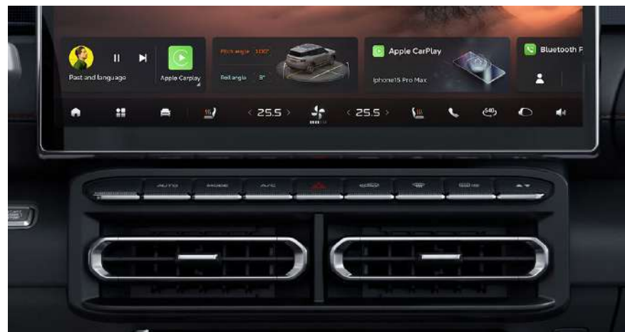
Dual-zone full automatic air conditioning
